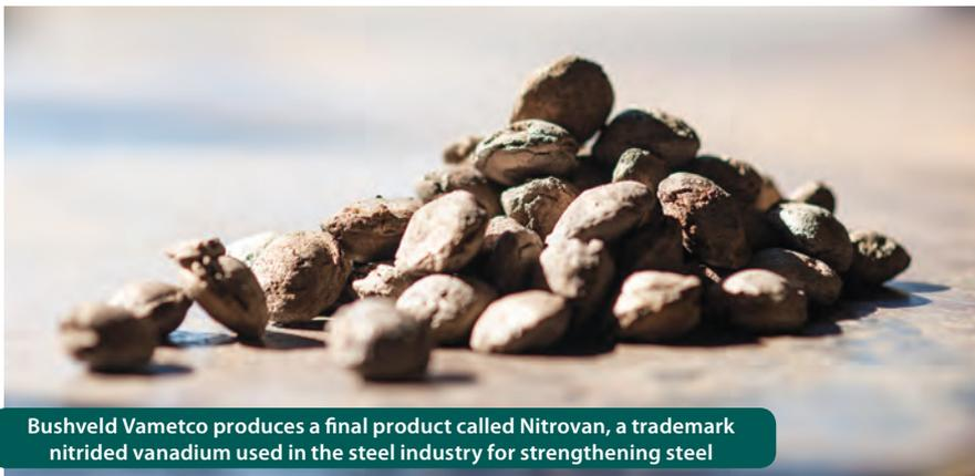
Bushveld Vametco produces a final product called Nitrovan, a trademark nitrated vanadium used in the steel industry for strengthening steel
